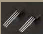
Uses FETs with carefully selected pair to match characteristics (700T common)
