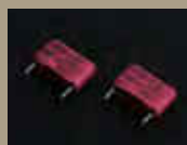
German WIMA Film Capacitor (700S Common)
